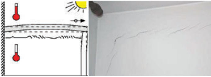
Figure 14: Cracking in masonry due to thermal movements of roof slabs Source: https://www.academia.edu/33589690/Defects_in_Masonry_Walls_Guidance_on_Cracking_Identification_Prevention_and_Repair
